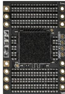
HIMALAYA is a discrete R2R DAC (digital-to-analog) module that is based on the FPGA algorithm. The combinations of its low audio frequency range, out-of-band noise, and low energy consumption make it a perfect match for high-performance audio equipment.
